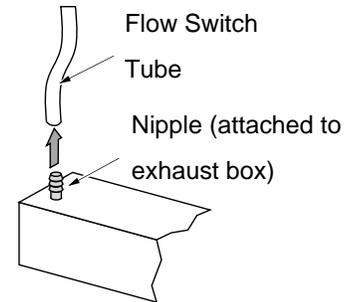
**(d)** Clean the blower blades, blower housing, and exhaust box. You may wish to use a vacuum to pull ash out of the vent system. When replacing the motor, take care to align the gasket (if it is damaged, replace). Check the nipple and flow switch tube. Insert a pipe cleaner through the nipple to dislodge any flyash. **NOTE:** The flow switch will shut off the auger if the tube becomes
