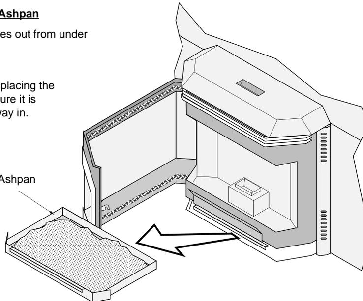
**Disposal of Ashes** – Ashes should be placed in a metal container with a tight fitting lid. The closed container of ashes should be placed on a non-combustible floor or on the ground, well away from all combustible materials, pending final disposal. If the ashes are disposed of by burial in soil or otherwise locally dispersed, they should be retained in the closed container until all cinders have been thoroughly cooled.
