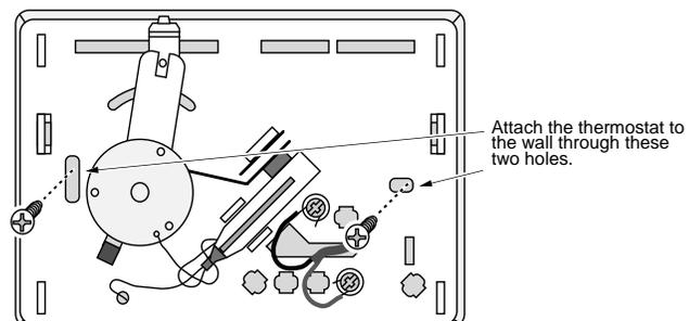
Attach the thermostat to the wall through these two holes.
