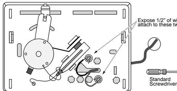
Expose 1/2" of wire and attach to these two posts.
