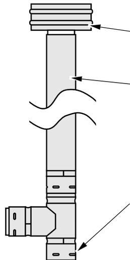
Make sure the cap is free of debris (especially if it has a screen that could become blocked).
