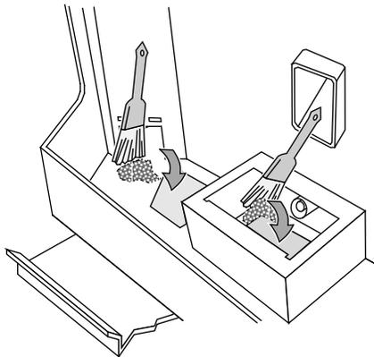
**g** Replace the ash trap doors and firepot. Slide the ash pan trap door forward.
